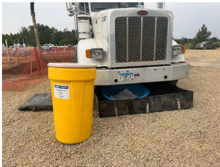
Facing east at MP 0.1, view of the hydro-vacuum truck in containment with the spill contained
